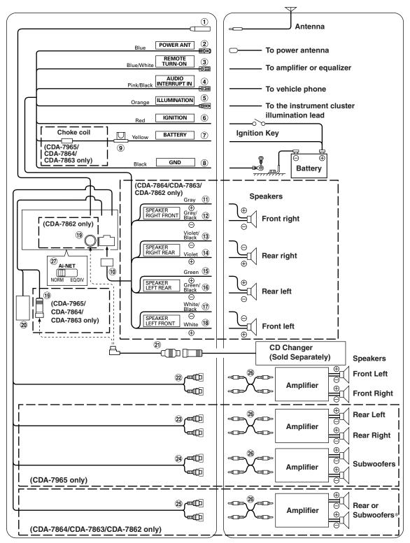
\* When Subwoofer is set to OFF: Output is from Rear speakers. When Subwoofer is set to ON: Output is from Subwoofer.
